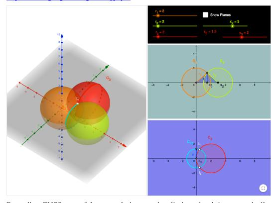
Regarding GNSS, one of the two solutions can be eliminated as it is geometrically incoherent. Nevertheless, a fourth satellite is necessary, as it provides solutions in the measurement of signal propagation time, due to desynchronization of the receivers' time compared to the satellites' atomic clocks.
